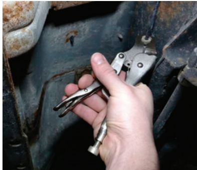
The OTC 6720 Flare Nut Locking Pliers removes rounded off nuts while saving the line.
